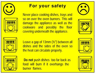
For the best results from the main oven we recommend that you use a baking tray which is 310mm (12") square. If you use a tray or tin which is larger than this, you may need to turn it around during cooking.
